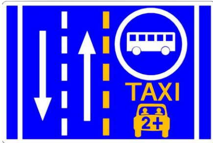
Image 4: Proposed traffic sign for lanes for public transport vehicles, taxi vehicles and vehicles carrying a minimum of two people
